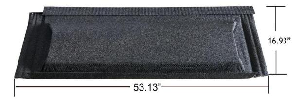
The WeatherLok Vent panel will install just like a normal panel. Lock it into place with the panel below it and use the five predrilled screw holes to secure it to the roof.
