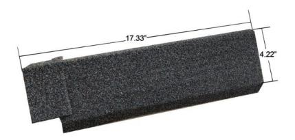
When the final top course of The WeatherLok Panel has been installed, the ridge cap should be installed. Using a 1 ½" screw, secure the first ridge Cap directly to the panel. Each piece of ridge cap will lock into the previous ridge cap. Each piece should be fastened on with screws through the overlaps.
